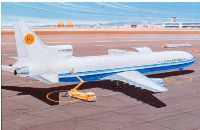
Figure 7 (upper left) shows an artist's concept of a Lockheed liquid hydrogen-fueled aircraft being refueled from two spherical LH2 storage tanks shown in the distance. Figure 8 (upper right) shows an advanced Lockheed LH2 fueled aircraft design that is fully optimized to take advantage of the use of LH2 fuel.
